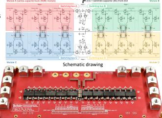
Photograph of the hardware prototype
